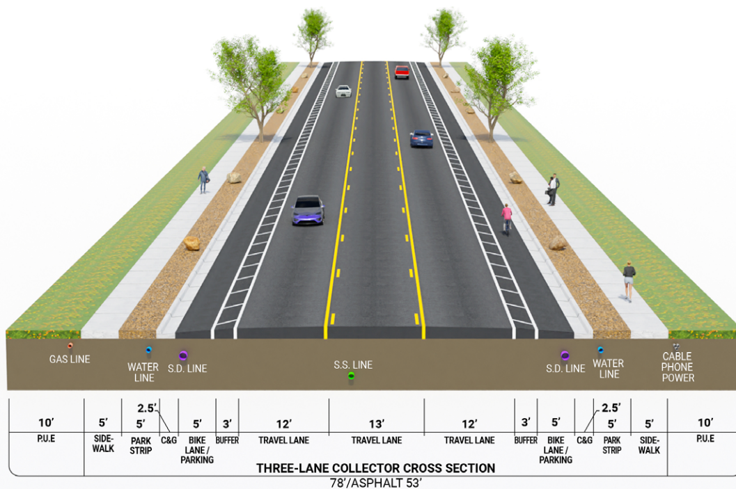
Figure 9: Three-Lane Collector Cross Section
