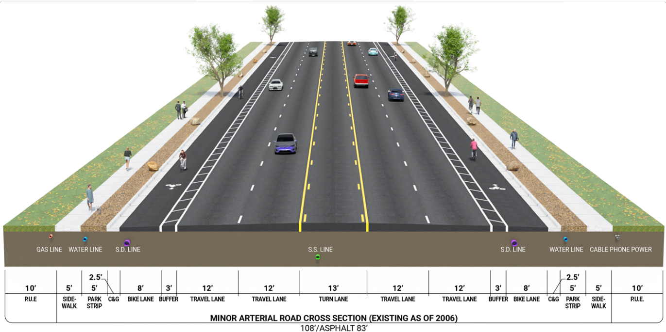
Figure 7: Minor Arterial Cross Section (Existing as of 2006)
